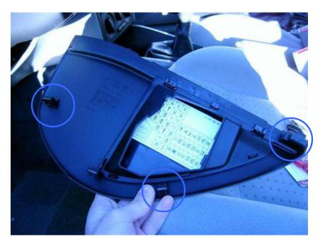
Now remove the plastic kick panel. It is held in place by 2 T20 torque screws:
