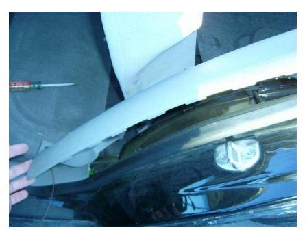
That piece is held in place by spring clamps that grip a metal strip. But at the top, it is held in place by something that doesn't just pull off So I just flexed the trim piece. Take care not to bend it though...
