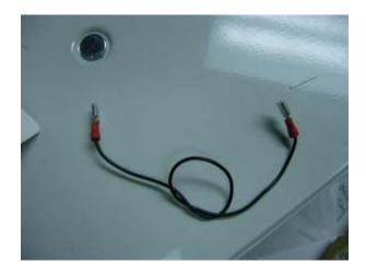
Cut the other piece of wire about 3/4 to one end. This is so that we can tell which way to plug it in when we get to the car 😇 Strip the ends in the middle, and melt some solder into them.
