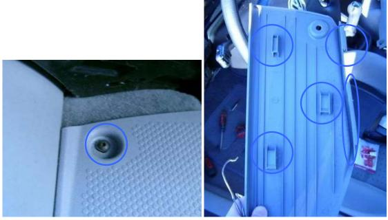
It was a real pain to get that thing off. With the screw out, it slides up and the 3 tabs on the 'face' disengage, but there are also 2 tabs that hold the pedal to the trim along the side of the car. You can see them in that pic. Just go slow, and don't try this when the plastic is cold and brittle I guess. For reference, here is what's under the dead pedal:
