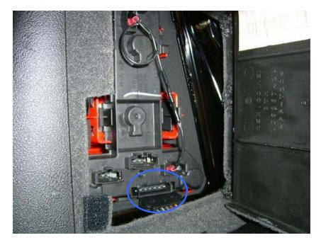
Disconnect the harness from the bottom of the socket assembly, as shown in the picture. It just pulls off.
