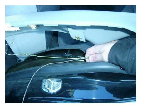
Take the hanger and push the wire all the way to the back of the car. Open the CD changer door, and the lamp access door. It will be above the tail light. It was kinda a pain to grab the wire, but I was able to. A helper might be good here to operate the hanger while you try to grab the wire. Construct the lamp access door is a suppose you could just try to push the wire back without using the hanger or fish tape... but I think it made life easier.
