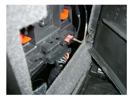
Woot! Driver's side is done! The passenger side is easier. Open the access door on the passenger side. Squeeze the clips again. The sockets are easier to get out on this side. Install a bulb in the empty socket. Run the jumper (the one without a diode.. the only one left hopefully) from the brake light pin to the rear fog pin. NOTE, this will be opposite of the way it was on the drivers side.
