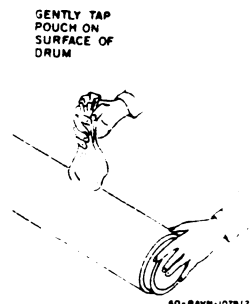
Figure 1. Lubricating the Drum
